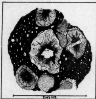
FIGURE 10. SPHERULITES AND MUD PELLETS IN FINE SHALY MATRIX. With abundant quartz fragments. Growth aprons of clear, light carbonate in the direction of extension. Fracture across center of spherulite healed with fibrous carbonate. Center of large spherulite is calcite. Three miles SE. Greencastle. Spec. 385.
